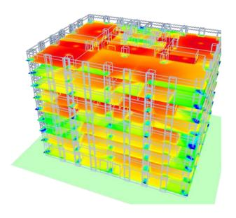
Heat map showing prediction of coverage of an inbuilding 4G(LTE) wireless network
